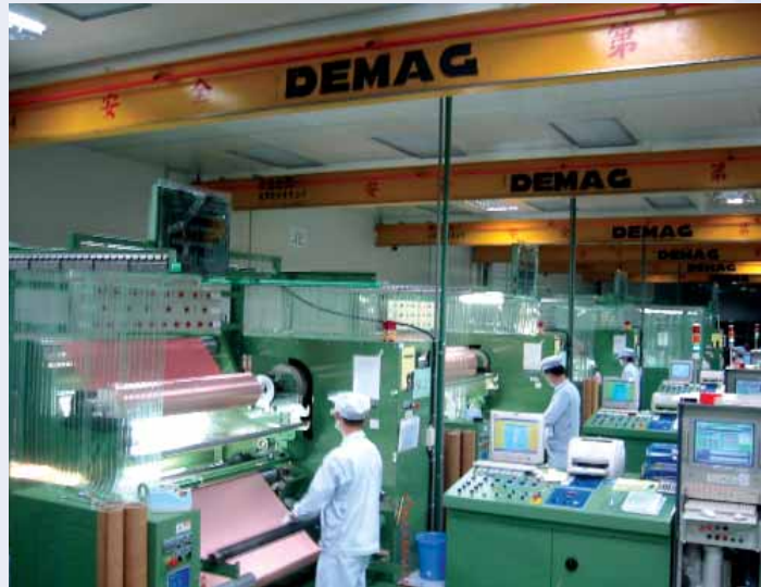
■ Copper foil inspection and cutting stations
